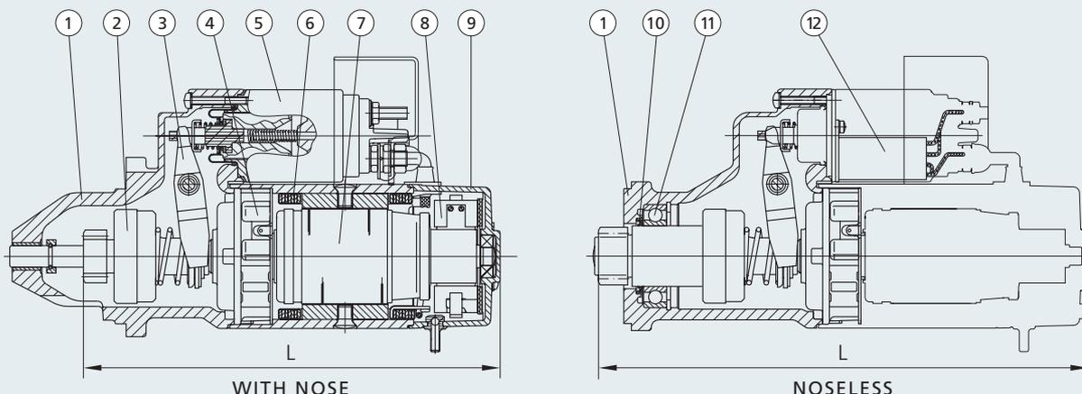
1. Drive end bracket • 2. Drive assembly • 3. Engaging lever • 4. Reduction gear • 5. Starter switch • 6. Stator
