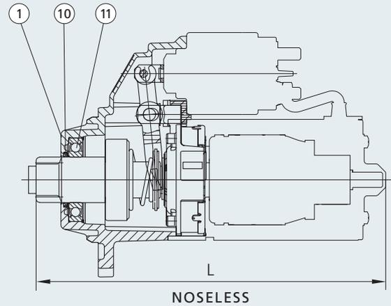
1. Drive end bracket • 2. Drive assembly • 3. Engaging lever • 4. Reduction gear • 5. Starter switch • 6. Stator
